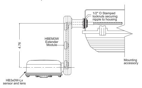
The  $\frac{1}{2}$ " chase nipple facilitates mounting through fixture knockouts, or attaching to threaded J-boxes or conduit hubs. An accessory bag with an 0-ring and two locknuts is available to accommodate various mounting needs. Mount the sensor so that the fixture does not obstruct the field of view.
