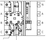
"Barrel" Shaped '7" Shaned Phase Connector Phase Connector
