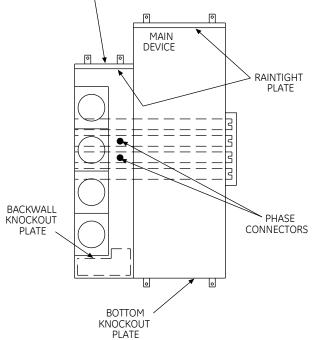
Fig. 4 Knockout Plate Locations and Phase Connections
