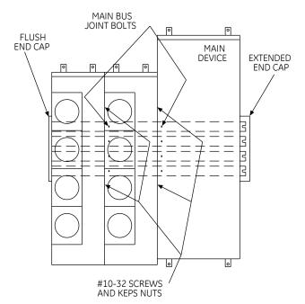
Fig. 3 Meter Module Assembly and End Cap Locations
