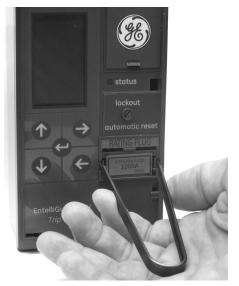
Figure 2. Rating plug removal
