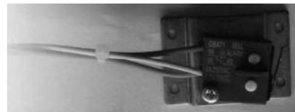
Bell Alarm with Lockout
