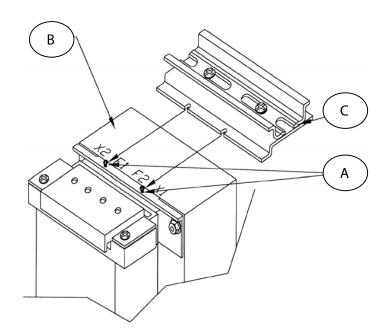
This kit includes parts that allow Hevi-Duty Control Transformers to use DIN mount protection devices for CE applications
