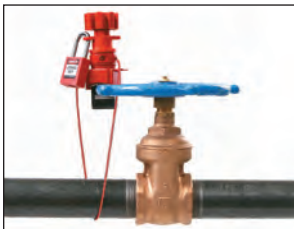
Use cable attachment to lock out gate valves.
