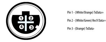
Figure 23 - I/O Receptacle Input Pinout (M12) - Female
