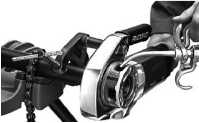
Figure 6 – Threading Pipe and Applying Oil
