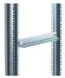
Equipment Guides help support rack-mounted equipment during installation. Guides mount between two pairs of rack angles. Slotted holes are provided for vertical or lateral adjustment. Furnished in pairs. Guides have plated finish. Mounting hardware included. Rack accessories that are shorter than the enclosure depth can be mounted to rack angles using Adjustable Rack-Mount Rails or Grid Straps. Order these items separately.
